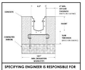
CONCRETE ENCASEMENT AND REINFORCING BASED UPON APPLICATION AND LOCAL CODES
