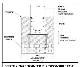
SPECIFYING ENGINEER IS RESPONSIBLE FOR CONCRETE ENCASEMENT AND REINFORCING BASED UPON APPLICATION AND LOCAL CODES
