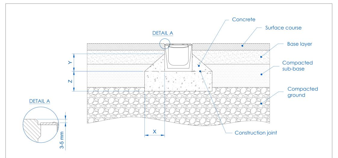
\* In case of an incorrect compaction of the soil, the concrete must be made up to the pavement level.
