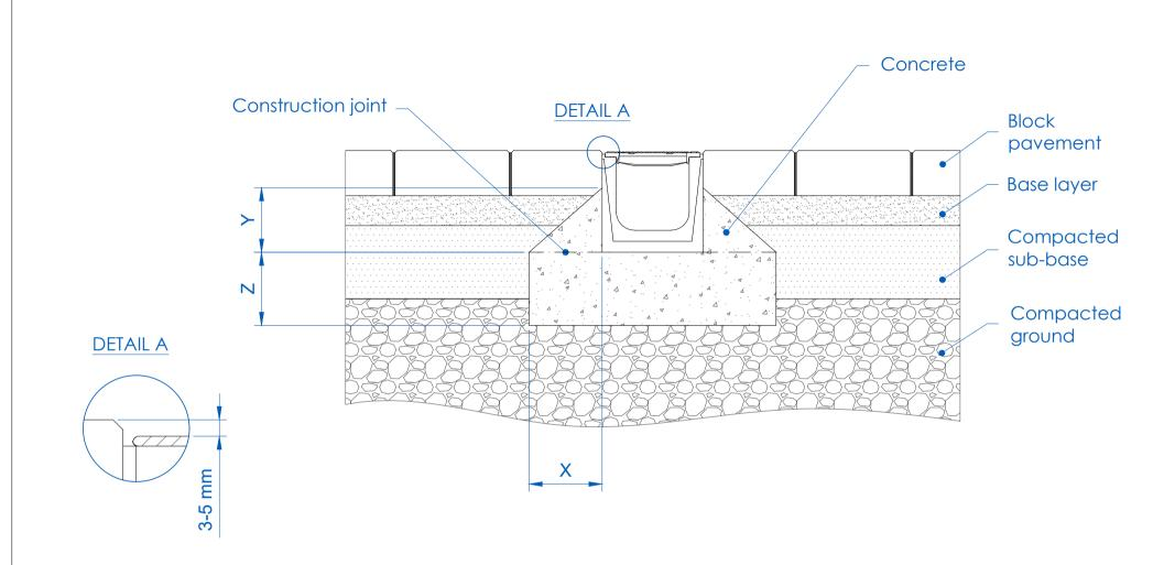
\* In case of an incorrect compaction of the soil, the concrete fill must be made up to the pavement level.
