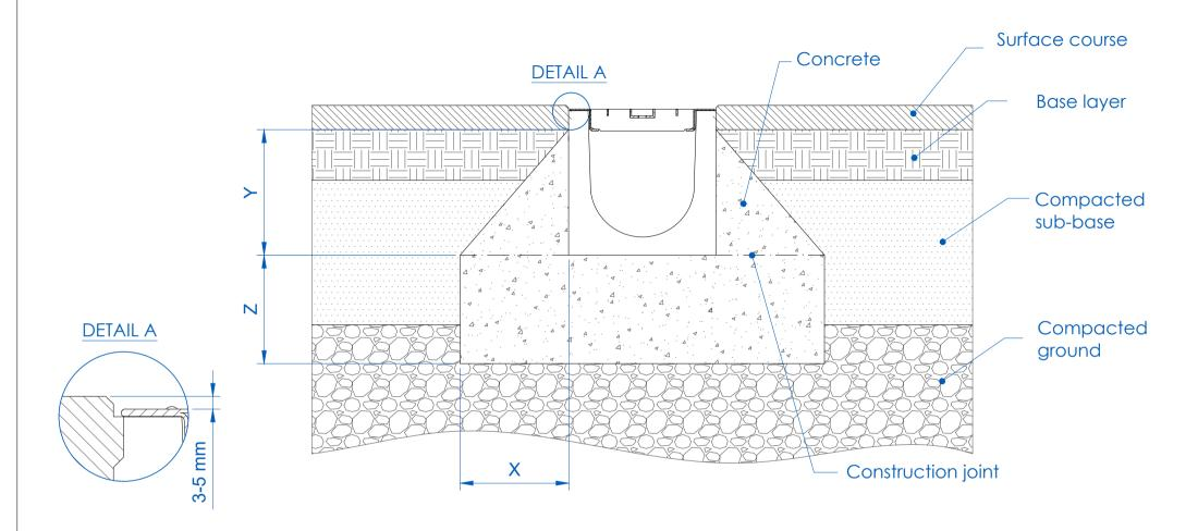
\* In case of an incorrect compactation of the soil, the concrete embracement must be made up to the pavement level.
