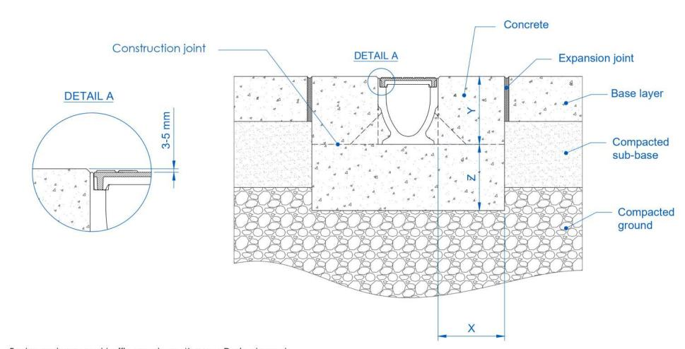
For heavy transversal traffic use always KompaqDrain channels.
