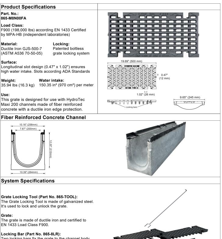
Two locking bars fix the grate to the channel body. They're unlocked by the Grate Locking Tool .
