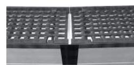
Joint tape may be required to close the gap between channels so concrete doesn't backfill into the channel during the encasement pour.
