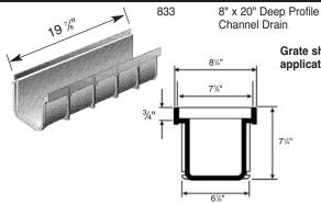
Profile high impact PVC channel drain with mechanical interlocking applications. Grate should be recessed 1/4" in traffic applications.
