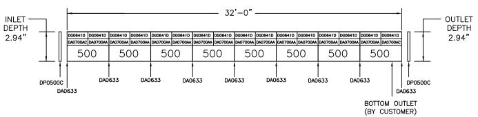
DRILL SIZE 3.50" FOR 3.0" SCH 40 & 80 PVC DRILL SIZE 4.25" FOR 4.0" SCR-35 SEWER & DRAIN DRILL SIZE 4.50" FOR 4.0" SCH 40 & 80 PVC
