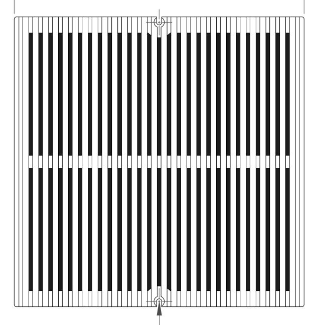
$2x \ 1/4-20$  counterbore slots for bolt-down to frame below
