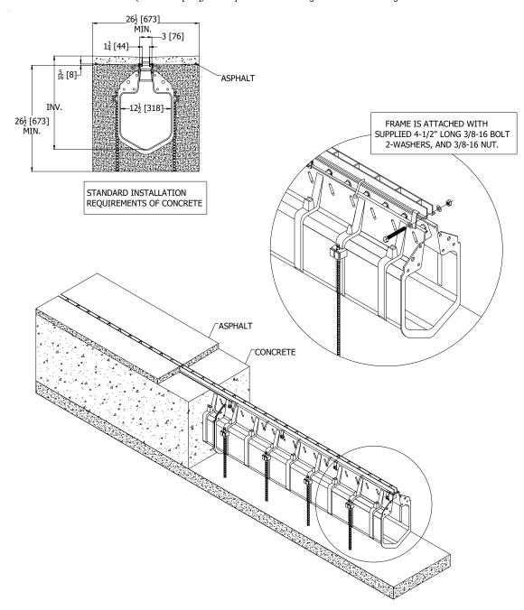
Our system can be installed with asphalt when using our special steel riser. It comes in two standard heights: 2" [50.8 mm] and 4" [101.6 mm]. Different heights are available upon request. The standard concrete installation is suggested around the Hi-Cap body for strength. A standard installation of the asphalt can be done up to a steel frame.
