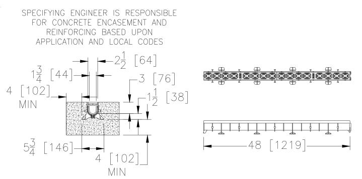
ENGINEERING SPECIFICATION: Zurn Z880 2 1/2 [64] Wide Trench Drain System shall be 48 [1220] long and 2 1/2 [63.5] wide. Drain shall be 3 [76] deep. Drain shall be made of (HDPE) High Density Polyethylene, and is UV-10 stabilized. Drain shall have bedding feet to be used for positioning and anchoring purposes. Drain shall have tongue and groove snap fit connection. Drain shall have 24 [610] long high-density polyethylene decorative grate (-POG) provided as standard.
