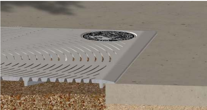
Close up section view of the retrofit tree grate. No frame required.
