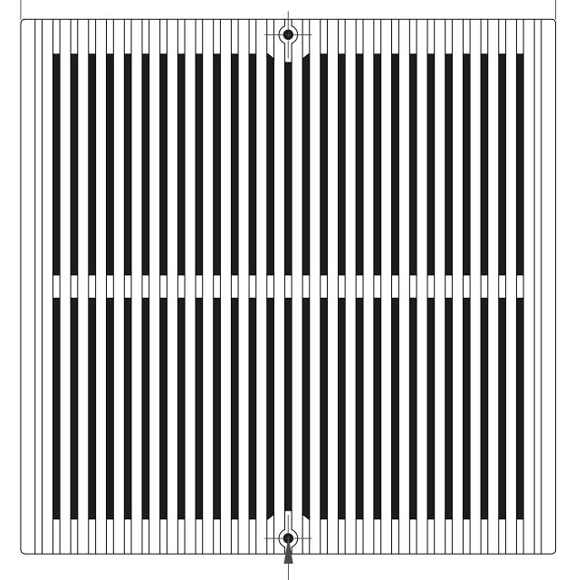
2x 1/4-20 counterbore — holes for bolt—down to frame below
