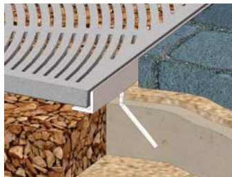
Standard for pavers – Eight standard 3/8" x 4" (10 x 102 mm) concrete anchor bars in frame used with pavers in surrounding area.
